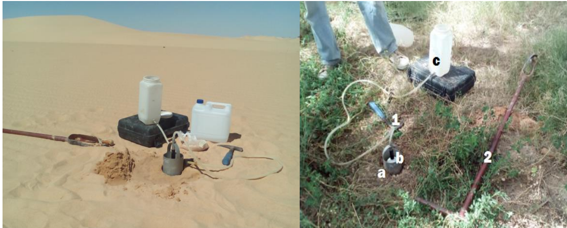
Photo 1: Viguiet permeameter installed at Erg (left) and Sebkha (right): (1) stainless steel level control cell (a), suspension device (b) (float), measuring tank (c), Auger (2).
