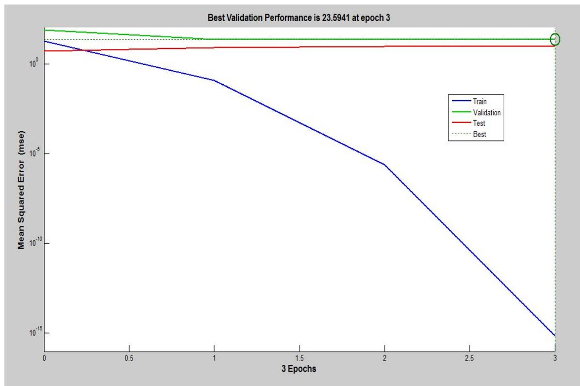
**Figure 3:** The train, validation and test curves response with respect to Epoch number, the goal was satisfied at 3'rd Epoch.
