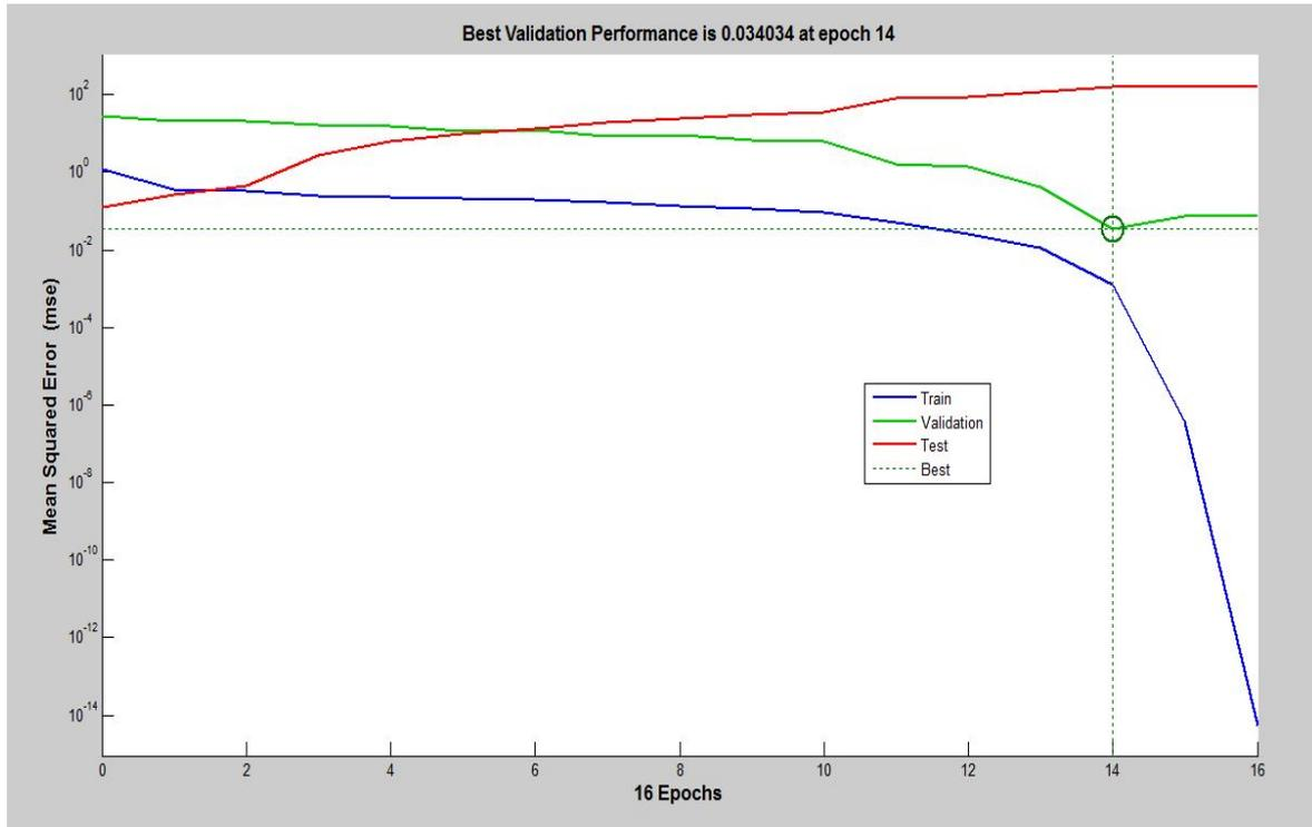
**Figure 4:** The train, validation and test curves response with respect to Epoch number, the goal was satisfied at 14<sup>th</sup> Epoch.
